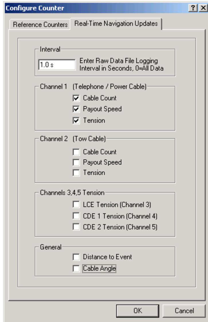
This dialog has two tabs. The first, **Reference Counters**, does not apply to this counter and should be left at the defaults. The second, **Real-Time Navigation Updates**, enables or disables this device's data from being passed to the vehicle. The three values available from this device must be placed into channel one. Uncheck all remaining values, as this counter does not read them.
